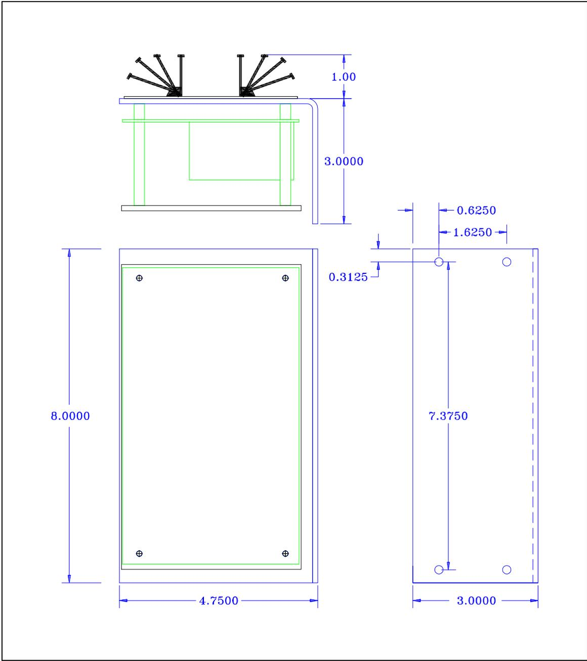
Figure 4 Dimensions of IBPS Power Supply
