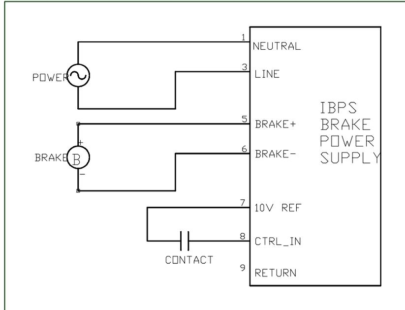
Figure 2: Simple Switched Control of IBPS
