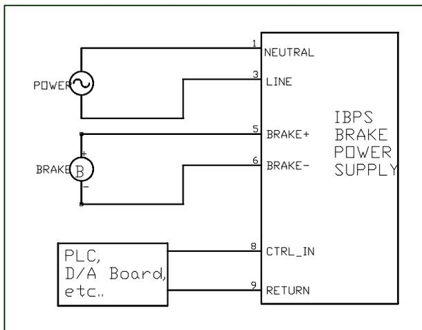
A simpler method of control where continuous control is not required, involves feeding the module's ten volt reference output back to the control input in **voltage control mode**. The amplifier's current would be adjusted via the span adjustment potentiometer on the board. The power supply could then be operated/controlled via an external relay or switching device.
